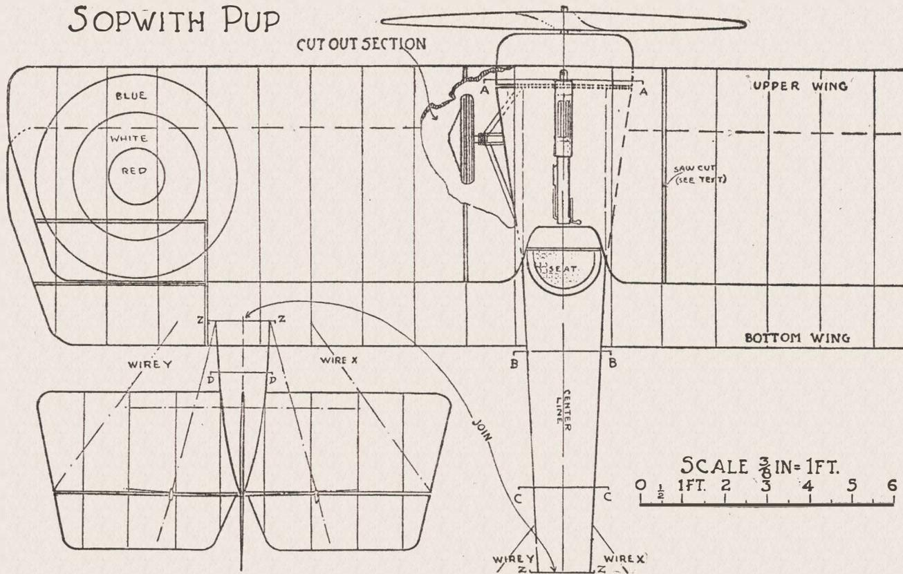
puts you up against a tricky bit of construction. There are two ways to construct the top wing. Either way calls for making the wing in one piece at first.
